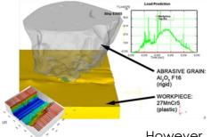
Grinding is the preferred choice for finishing automotive gears and rotors because of its high productivity and capability to machine heat-treated or brittle parts with high geometric accuracy and surface quality. Material removal processes for rotors' permanent magnets are particularly challenging due to their high hardness and brittleness, and the grinding process is crucial for reaching the dimensional tolerances requested by the product.
